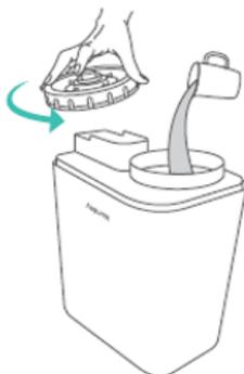
4. Fill the water tank with water, screw the water tank cap back in place and securely place the water tank back onto the base. The water tank level can be viewed through the window on the left-hand side.
